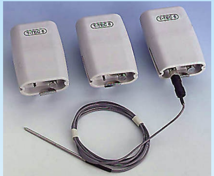
Three T-TEC 6 data loggers, internal sensor; fixed external sensor and remote sensor.
