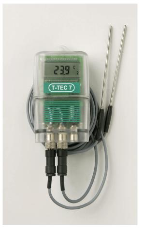
Thanks to the unique casing in clear polycarbonate it is possible to have a large display and watertight qualities as well. Actual temperature is displayed constantly. When the T-TEC 7 is set up for datalogging, a logging indicator is turned on. When the logging starts, the indicator will flash with 4 seconds intervals. Triggered alarms will flash with 4 seconds intervals, alternating with the temperature display.
